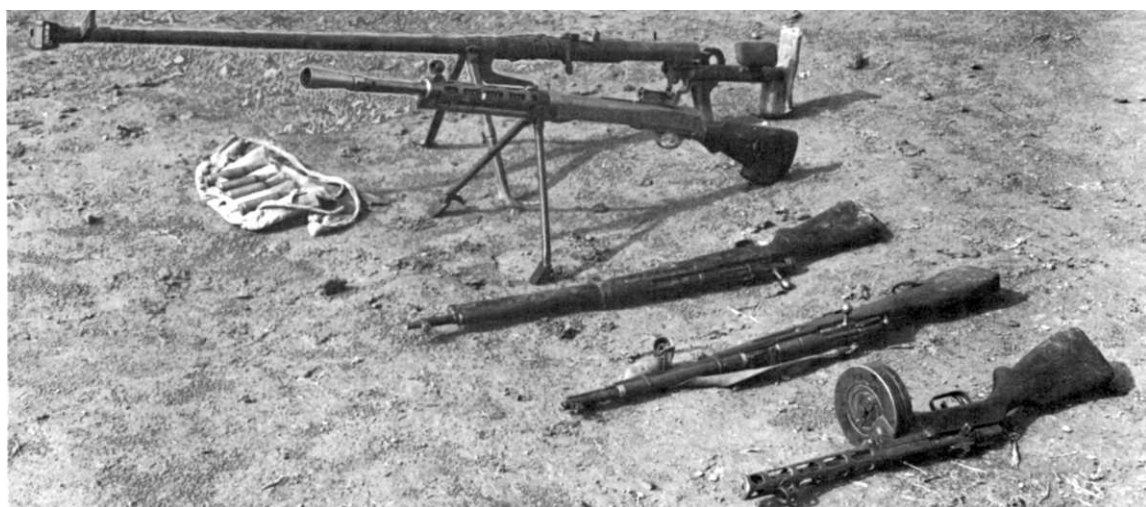
Small arms (front to rear): Russian 7.62-mm. submachine (burp) gun; Russian 7.62-mm. carbine M1944; Japanese 7.7-mm. rifle; Russian 7.62 Tokarev semiautomatic rifle with flash hider; Russian 14.5-mm. antitank rifle PTRD-1941 (Degtyarev).
